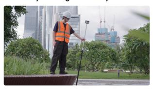
The V10i supports the Tilt Survey of 60 degrees. We don't need to hold the survey pole upright when measured, which improves the efficiency of the measurement. When we meet some positions where we can't hold the pole upright, the Tilt Survey function will help you solve it easily.
