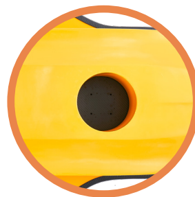
ADCP access shaft
